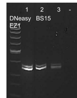
Figure 6: Amplifications (25 µl reaction volume) were performed using the avian CHD PCR system* with 2 µl eluted DNA (from 5 µl blood) from 3 different chicken and systems. PCR products (3.5 µl) was visualized on a 3% agarose gel. The marker was 30 ng 50 bp std. "-" is negative control.
